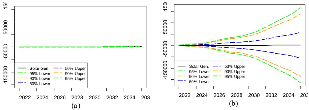
**Figure 4.2.3.2:** Uncertainty cones for solar net generation (billion kwh), on the same scale, for (a) method  $G_1$  and (b) method  $G_2$
