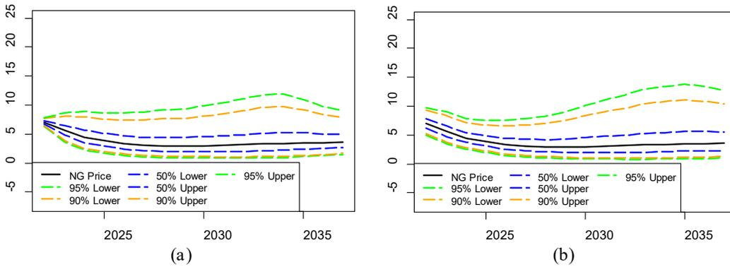
**Figure 4.2.2.4:** Uncertainty cones for projected natural gas prices to the electric power sector (dollars per million Btu) computed by (a) method  $G_1$  (b) estimated method  $G_1$
