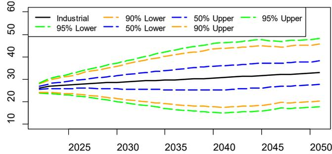
**Figure 3.2.1:** Gaussian uncertainty cones for industrial energy consumption (quadrillion Btu), estimated based on historical volatility (method  $G_2$ )
