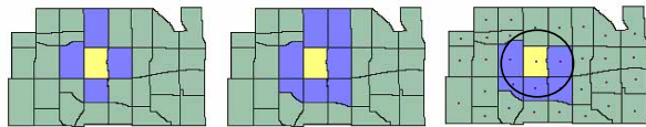
Figure 1: Different methods for defining neighbouring regions for the selected region in yellow. A) Rook contiguity – includes locations with a common border, B) Queen contiguity – includes regions with a common border or vertex, and C) Distance – includes all regions whose centroid is within the specified distance band.
